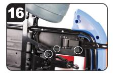
Secure the cable cover carefully to the chassis using the 3 screws removed before. Make sure not to pinch the wires.
