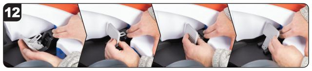
Holding the black pedal base in place, push the new pedal towards the pedal base and feed the gray strip (on the back of the pedal) into the open slot until it clicks.
