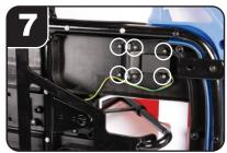
Being careful to avoid pulling or damaging the green and yellow wires, remove the 6 screws from the chassis shown above, and set the 6 screws aside.
