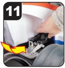
Install the new pedal in the same position as the old pedal.
