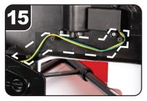
Carefully position the wires flat against the chassis, threading the wires as shown above: under the left plastic post, over the middle plastic post, and under the right plastic post.
