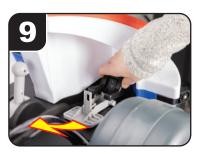
Gently lift the black pedal base (no more than 1 inch). Remove the old pedal (gray portion only) and put it aside.
